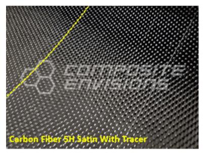
If material tracers are not an option and fiber orientation is not visually obvious while laying up, a given ply can be marked with a layup approved pen. A "Pentel White 100WS" will mark plys and provide a simple reference line to follow through a layup process. It should be noted to not put this on the first or last ply, as it may show on the final part. This ink will not degrade the fiber properties or the resin's ability to bond with the fabric.
