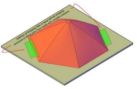
process. These tabs can be made from the extra plies in the layup or fiberglass just lying around. Place these plies in an excess area beyond the part's final trim line, and there will be
