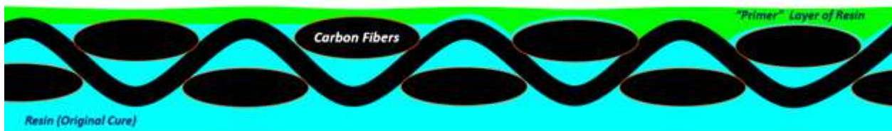
Additional Layer of Resin provides numerous benefits before application of clear coat
