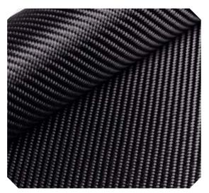
however, as it transfers that energy along its fibers to other sources. This may be good or bad dependent on application. Carbon Fiber is best used with epoxy resins to achieve its maximum properties. Although special tooling and processes are not needed for fabrication purposes, vacuum equipment will greatly increase Carbon Fiber's laminate quality.
