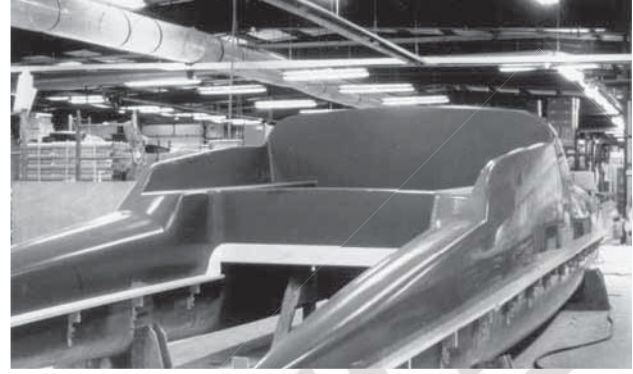
Figure 3-3 The catamaran plug was faired and finished to the same degree as the finished product. The shelf was applied to the plug where the mold halves divide the form at its widest point.
