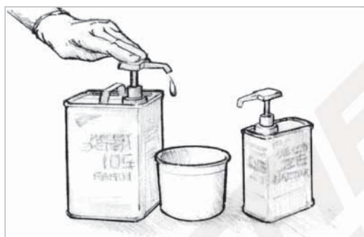
Figure 5-4 Dispense the proper proportions of resin and hardener.
