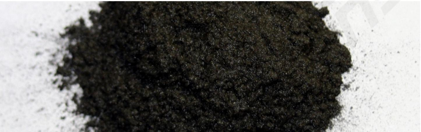
**Carbiso™ MF is recycled carbon fibre milled to 80µm or 100µm.**
