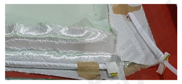
3. To connect the MTI® hose with the vacuum pump we recommend a 3/8" OD solid hose which is plugged into the spiral tube that is inside the MTI® hose. Pull the membrane sleeve over the joint and seal with sealant tape. Be accurate with the sealing operation to prevent resin from entering the vacuum line.
